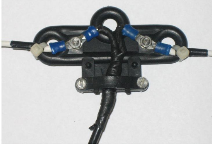
**Figure 7 - Dipole Centre Piece**
